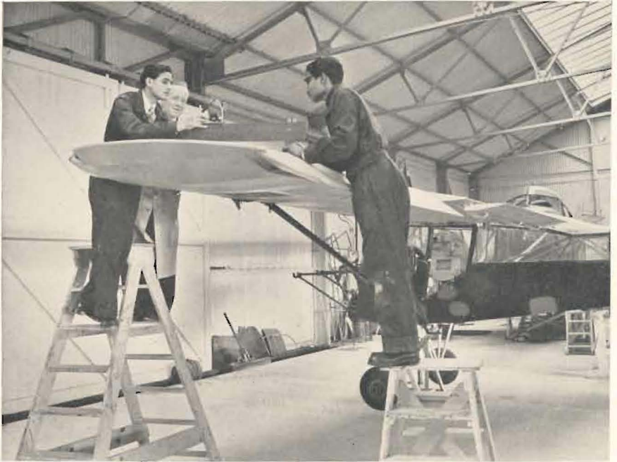
An Air Service Training instructor supervises a wing incidence check on an Auster Mk. 6.
